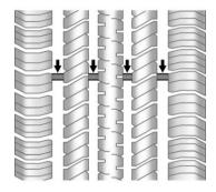
One way to tell when it is time for new tires is to check the treadwear indicators, which appear when the tires have only 1.6 mm (1/16 in) or less of tread remaining. See *Tire*  Inspection on page 10-79 and Tire Rotation on page 10-79 for additional information.
